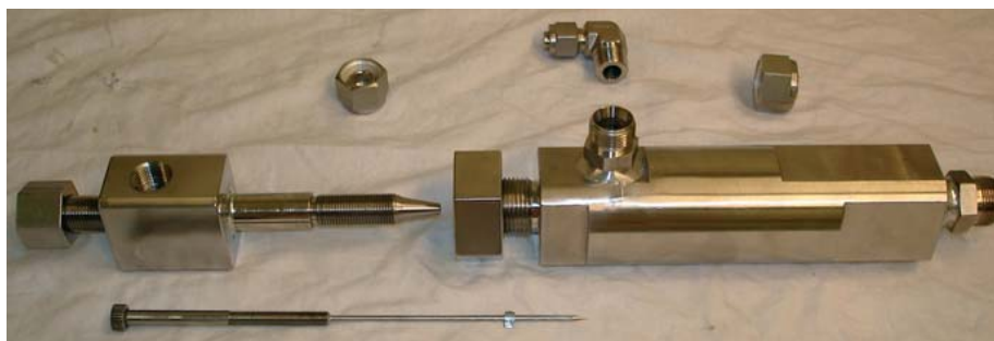
Figure 6: Photograph of controllable ejector expansion device
